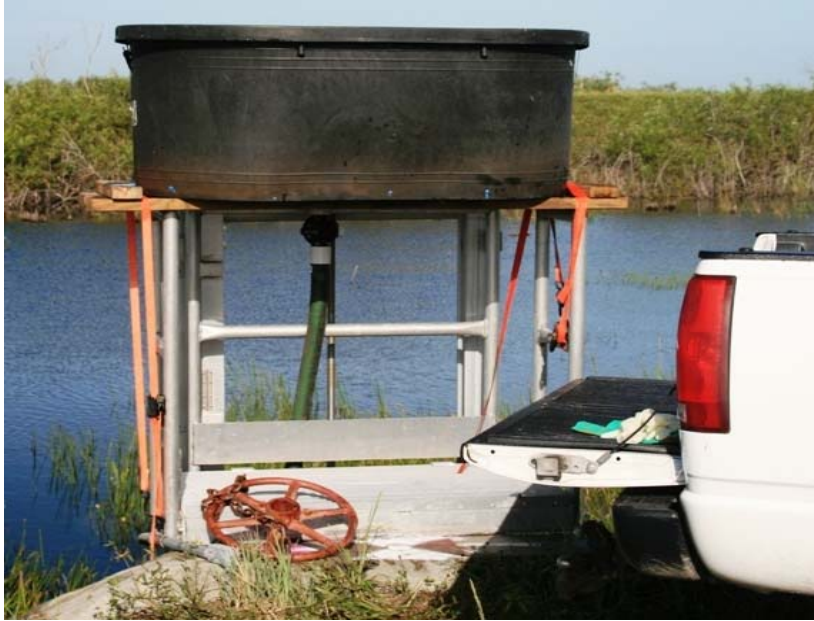
Figure. 6.2.5.2. Dye injector - note valve below mixing tank that allows for constant flow.
